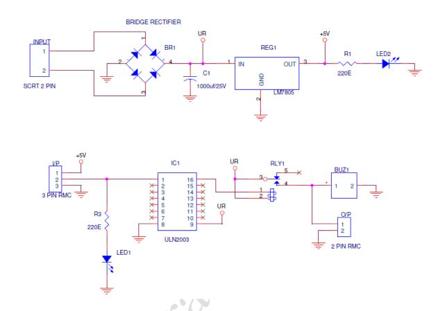
This project about Motion Detector based on PIR sensor. When any moving object is detected around 180 degree of PIR sensor, an active high signal triggers the LED strip ON via Driver unit ULN2003 for the time period of 15 sec and start continuing sensing next motion. The whole circuit Requires Regulated +5 V DC source, supplied by Bridge rectifier, filter capacitor and 7805 regulator.
